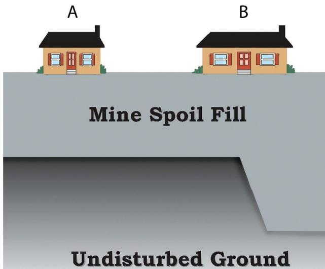
**Figure 1.** Settlement of underlying mine spoils can affect buildings constructed on mine-spoil fills. The spoil depth under building A (left) is relatively uniform, whereas building B (right) is built over an area where spoil depth varies. Building B is more likely to be damaged by differential settlement because it covers a larger lateral area and because of variations in the depth of the underlying spoils.
