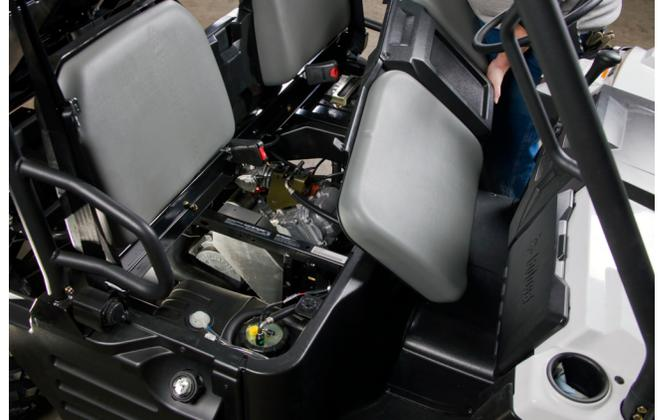
Liquid-cooled engine with radiator under the seat.
