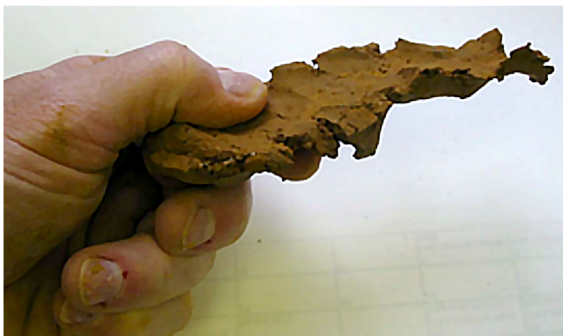
Figure 5: Guide to estimating one of 12 texture classes by hand from a moist, mixed soil sample about the size of an egg. This sample makes a ribbon over 4 inches long and is not very gritty, and would be classified as a clay, or silty clay, depending on how much grit could be felt. Photo courtesy of John Galbraith, Virginia Tech.
