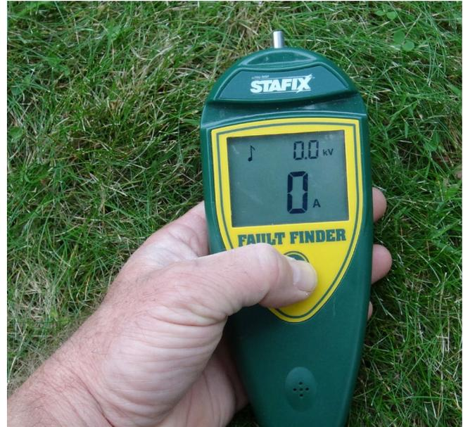
**Figure 1.** Voltmeter/fault finder. Image source: Matt Booher.
