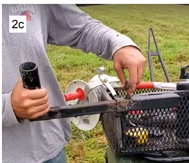
2c and 2d. An adjustable metal tube arm mounted on the front rack of this four-wheeler serves to hold a reel for hands-free unrolling of temporary wire.
