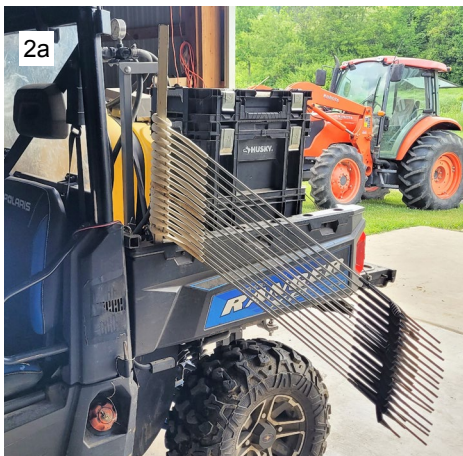
2a. A removable post mounted on an ATV provides a tangle-free way to carry pigtail posts.
