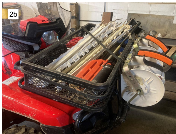
2b. A front-mounted rack on a four-wheeler aids in carrying posts, reels, and other temporary fencing tools.
