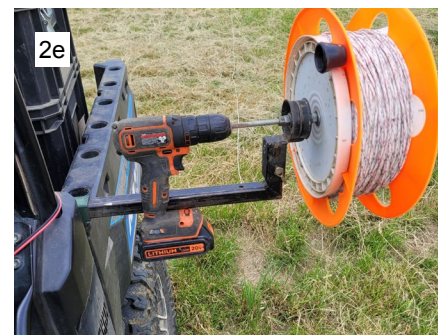
2e. A standard extension cord reel adapted for use with a battery-powered drill eliminates the need to reel up poly wire by hand.
